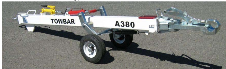
A380 Towhead Assembly ( to be used with PSE-170H Heavy Duty Towbar Assembly)
